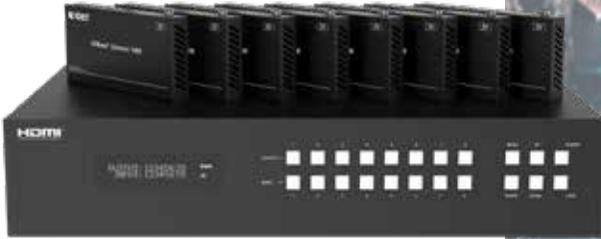
Front panel with OLED screen and supports control via front panel buttons, IR remote, RS-232, LAN, and Web GUI.
