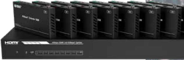
IMOWARE HDB800-4K-150 is a controllable Splitter and can distribute 1 HDMI sources to 8 displays. The resolution is up to 4K2K@60Hz 4:4:4, 18Gbps and HDCP 2.2. Each HDMI output supports 4K2K to 1080P downscale independently. The IR signal follows HDMI video channel at the HDBaset Receiver end. The product supports control via RS-232.
