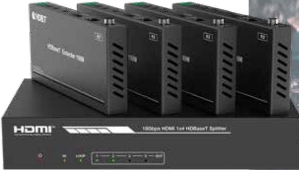
IMOWARE HDB400-4K-150 is a controllable Splitter and can distribute 1 HDMI sources to 4 displays. The resolution is up to 4K2K@60Hz 4:4:4, 18Gbps and HDCP 2.2. Each HDMI output supports 4K2K to 1080P downscale independently. The IR signal follows HDMI video channel at the HDBaset Receiver end. The product supports control via RS-232.
